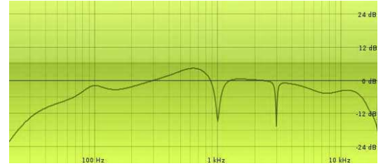
An EQ curve with two frequencies notched out. Even if this would get rid of room tone, it would also degrade the sound of your voice tracks.
